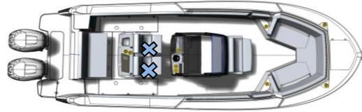
\* Ballast used to simulate weight of full fuel and water tanks and located on deck over fuel tanks
